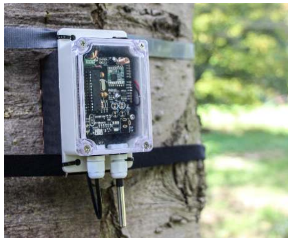
Figure 6. Application: the proposed platform is employed as a sensor for monitoring the health of trees.
