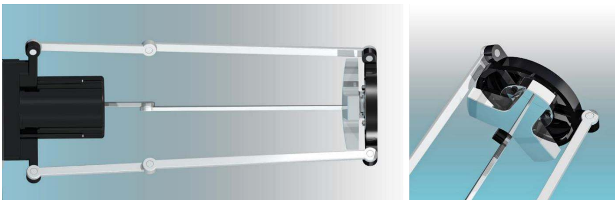
Figure 8.6: Secondary Mirror and its support deployment mechanism
