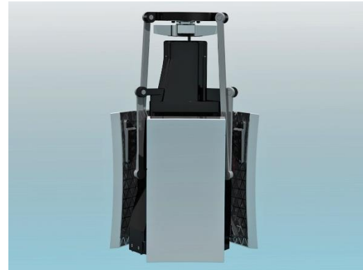
Figure 8.9: Deployable Telescope in the stowed configuration
