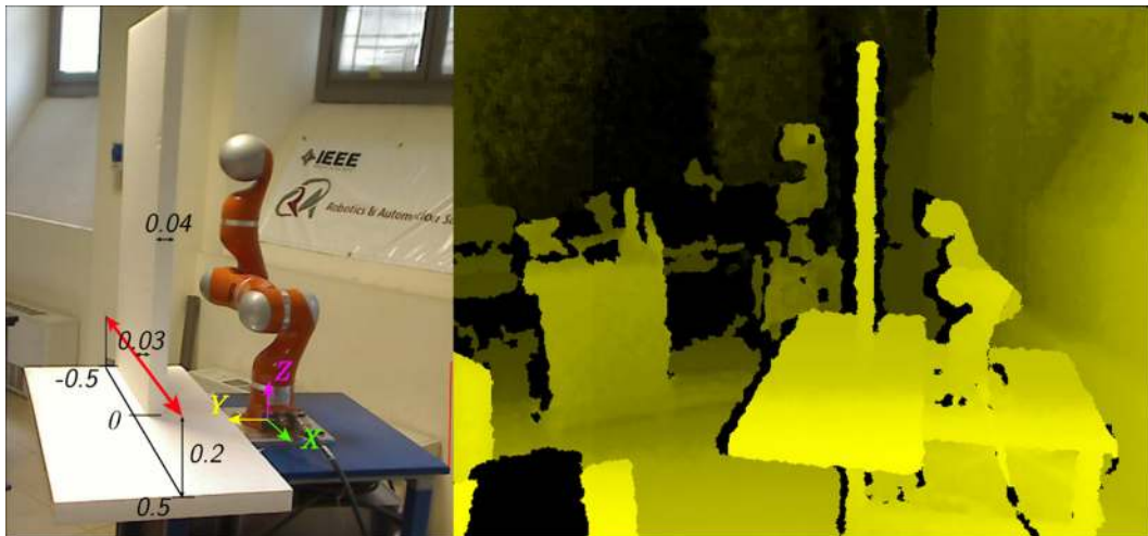
Fig. 6 Environment used for validation and comparison of methods. The virtual control point moves on the red segment shown in the left picture, while the depth image given by the
