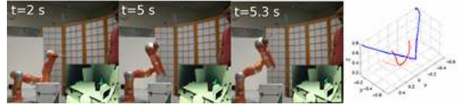
Fig. 14. Experiment 3: Image flow (on the left) and end-effector (in blue) and elbow (in red) trajectories (on the right) when all moving parts of the robot are considered for collision avoidance. The dashed lines in the plot represents the motion in the absence of obstacles
