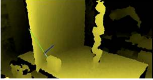
Fig. 5. Example of repulsive vector computation. Lighter colors refer to obstacle points with smaller depth, the point of interest \mathbf{P} is represented by a red circle, and the minimum distance is represented in cyan. The repulsive vector obtained by using the minimum distance only is shown in green, while the one obtained by using all points in the range of surveillance is in blue. It can be seen that the green repulsive vector points to another obstacle (dangerous), while the blue vector points to a free area (safer)
