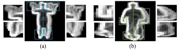
Fig. 6. Spatiotemporal body parts motion features based on maximally confident patches in case of (a) both hands waving and (b) walking activities using our depth annotated dataset.
