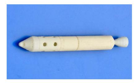
Figure 149: 3D model of a slender-body vehicle
