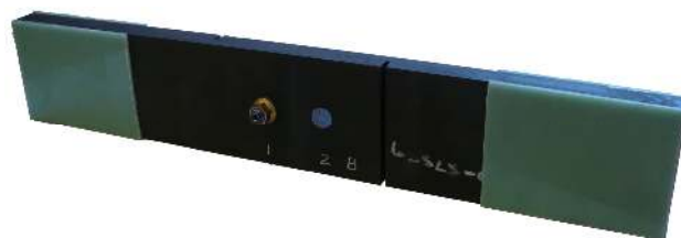
Fig.1. Specimen of a composite bolted joint for the experimental unsupported single lap shear test.
