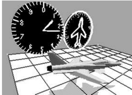
Figure 8.10: Gauges serve as both displays and controls of the plane’s configuration. Although they are 2D objects, the gauges can be placed anywhere in the 3D scene.
