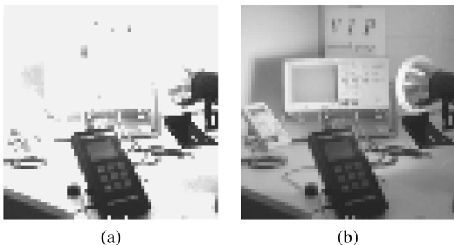
Fig. 12. Wide dynamic range image capture. (a) Image capture using a linear ADC response. (b) Image capture with the nonlinear ADC response.
