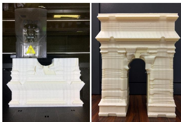
Fig. 10: The model during the 3D printing and at the end, surrounded by support material.
