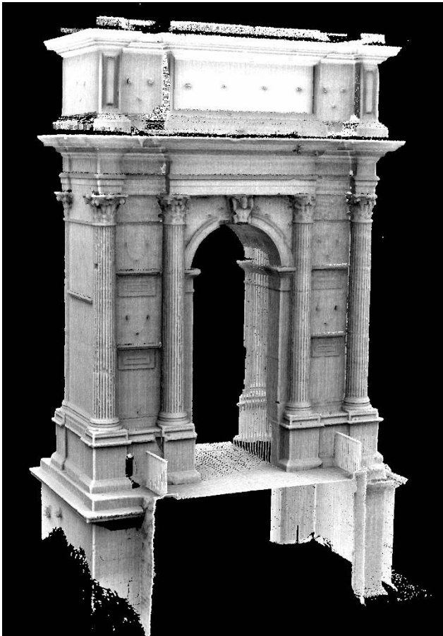
Fig. 3: Point clouds obtained from TLS survey
