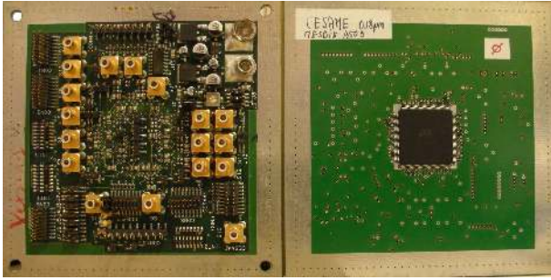
Fig. 6. ALI board (left: connector side, right: IC side)
