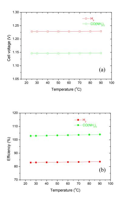
**Fig. S1 (a)**, Theoretical cell voltage of fuel cells,  $H_2$  ( $\Box$ ) and CO(NH<sub>2</sub>)<sub>2</sub> ( $\bigcirc$ ). (b), efficiency of fuel cells  $H_2$  ( $\blacksquare$ ), CO(NH<sub>2</sub>)<sub>2</sub> ( $\bigcirc$ ).
