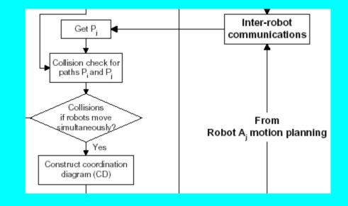
All these mappings are combined into an N-dimensional coordination space represented by a *coordination diagram*.
