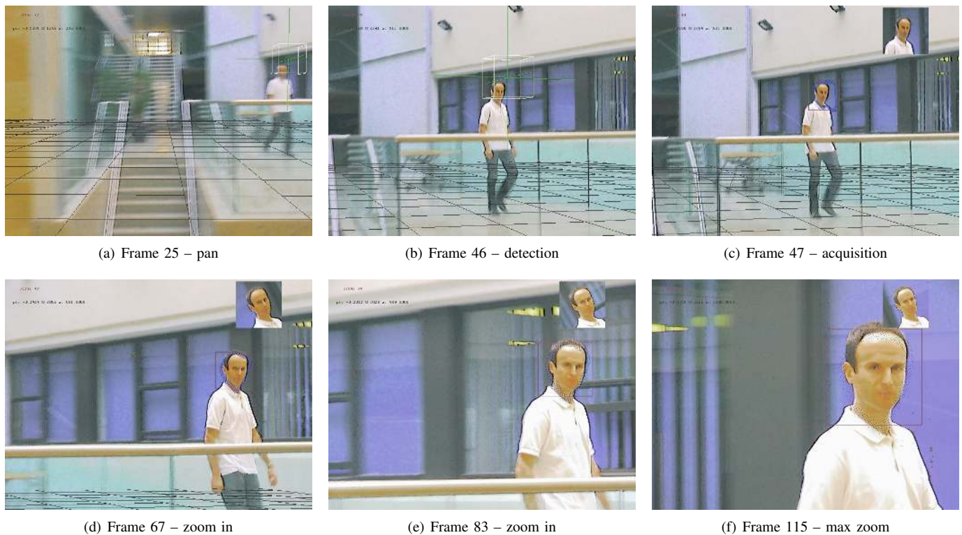
Fig. 7. Multi-resolution tracking over long distances. Zoom factors are changed from 1 to 2.5 in frame 25, 4.5 in frames 46 and 47, up to 10 in frame 115. Note the stabilised closeup image in the upper right corner once the target is acquired, and which is stored in the database. To speed up initial acquisition of the target, the active tracker is not always run until full convergence (see face boundary in 47). This can result in subsequent rotation of the closeup image.
