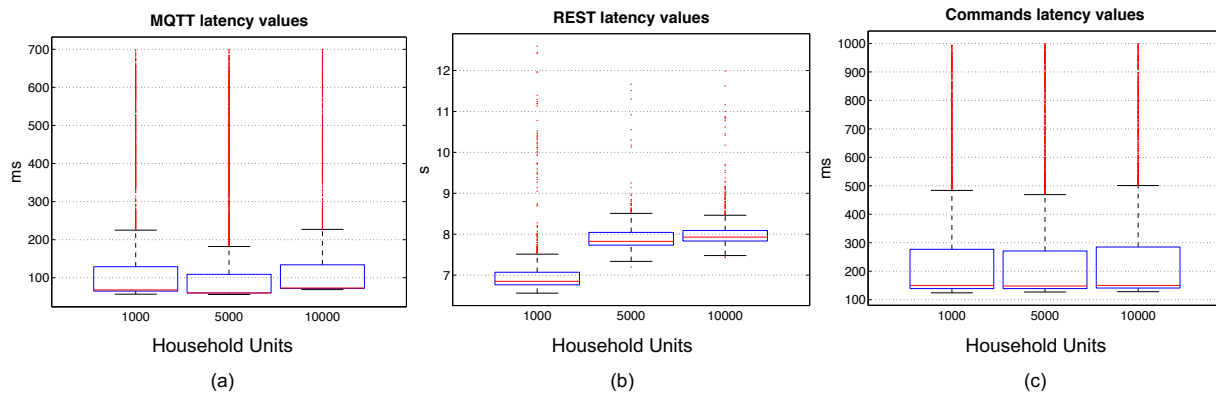
Fig. 11. Transmission latency at different Household Units: (a) MQTT, (b) REST, (c) Commands.
