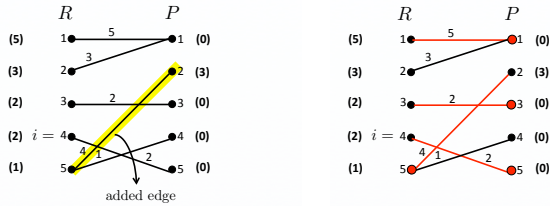
(a) Step 2: For the updated y , the corresponding set of equality subgraph E_y (with the new, added edge highlighted in yellow). (b) Step 2 contd.: For the updated E_y , a maximum cardinality matching edges M_y (red edges), and a corresponding minimum vertex cover V_c = (R_c, P_c) (red vertices).
