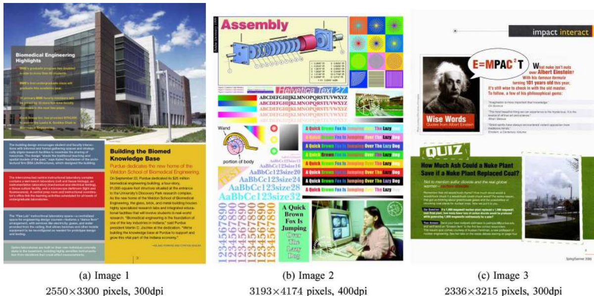
Fig. 8. Thumbnails of the original test images. The corresponding JPEG encoded images have bit rates 0.43 bits per pixel (bpp), 0.53 bpp, and 0.32 bpp, respectively. All the three images were compressed with 2:1 chrominance subsampling in both vertical and horizontal directions.
