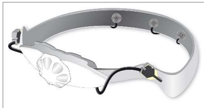
FIGURE 1 | Sketch of the prototype dry electrode cap. The three comb-like electrodes are placed inside in the back of the cap. Ground and reference are placed laterally in the front. Moreover, there is a wheel to tighten the cap to the participants’ head.
