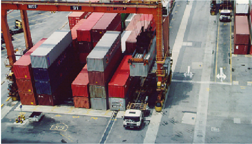
Figure 2. An RTGC spans the width of a block with seven rows of spaces between its two legs. Six of these rows are used for container storage, the seventh (rightmost in the figure, a parked truck is in the row) is for truck passing.
