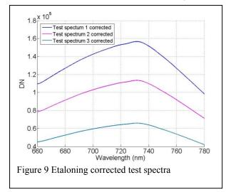
wavelength interval. This confirms that this curve fitting, residual interpolation and look-up table correction process achieves a significantly more accurate correction of etaloning than was achieved using the 'referencing' approach. It also demonstrates that QE Pro spectrometer etaloning can be successfully corrected in a post processing procedure.
