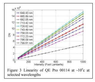
1,000fl, close to Ocean Optics' automatic integration maximum setting of 85% of 180,000 counts [7]. It is acknowledged that it is not possible to de-convolve etaloning linearity and detector linearity by this method. Nevertheless, it is the system's linearity that is key to making accurate measurements and it is the system's it
