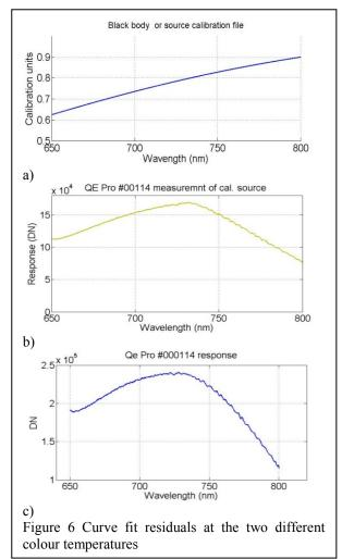
was again used. The QE Pro was set: to average 30 measurements; integration time to achieve 160,000 counts, dark current subtracted; and non-linearity correction enabled. Measurements of the source made at 20 levels of intensity. Three of these were selected to assess the method and the remaining 17 used to develop the correction method.
