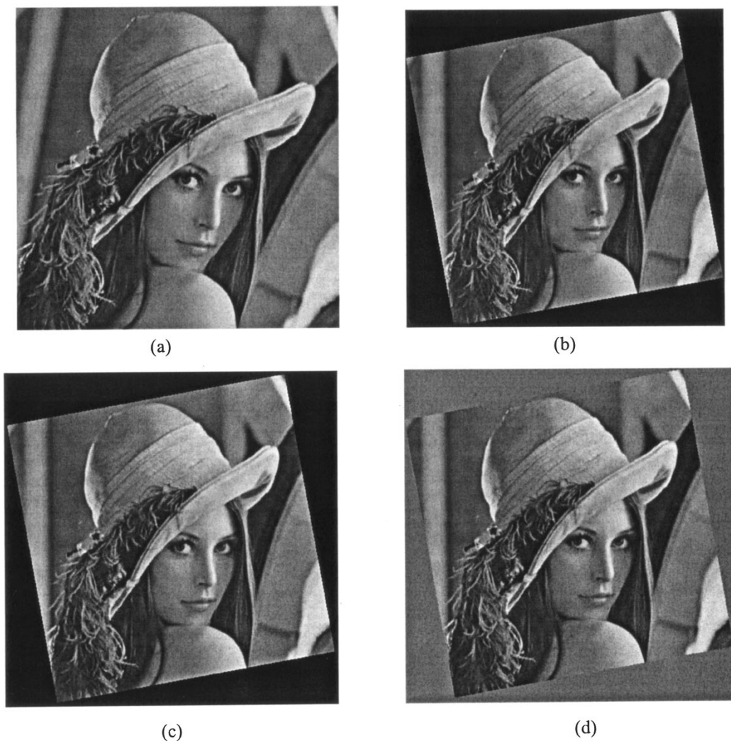
Fig. 6. Resynchronization: (a) the to-be-checked image g(x, y) , which is of 512 \times 512 and is experienced a rotation of 10^\circ , scaling, translation, cropping, and JPEG compression with quality factor of 50; (b) the image g'(x, y) , which is of 504 \times 504 and has been recovered from the linear transform applied; (c) the image I(x, y) , which has been padded with 0s to the size of 512 \times 512 ; and (d) the resynchronized image g^*(x, y) , which is of 512 \times 512 and has been padded with the mean gray-scale value of the image g(x, y) . The embedded message was finally recovered without error.
