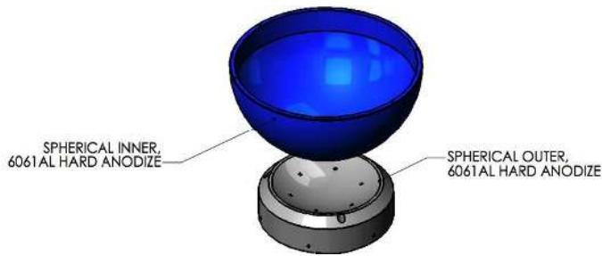
Figure 6. Aluminum hemisphere with air-bearing by Nelson Air Corp.
