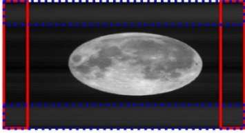
Fig. 11. Signal selection for estimating dynamic dark level. The static dark level value is estimated by the mean value of signals inside the red box. The time variation model of the dark level is established by signals inside the blue dotted rectangle.
