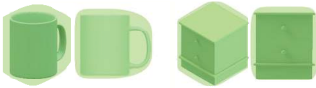
Fig. 9 Illustration of two complex objects that are modeled with two smooth hyper-surfaces. The analytical model for the drawer is \Gamma(\bar{\xi}) : (\bar{\xi}_1/0.4)^4 + (\bar{\xi}_2/0.4)^8 + (\bar{\xi}_3/0.6)^4 = 1 , and the mug is modeled with (\bar{\xi}_1/0.05)^4 + (\bar{\xi}_2/0.05)^8 + (\bar{\xi}_3/0.05)^4 = 1 when \bar{\xi}_2 > 0 and (\bar{\xi}_1/0.05)^4 + (\bar{\xi}_2/0.08)^2 + (\bar{\xi}_3/0.05)^4 = 1 elsewhere.
