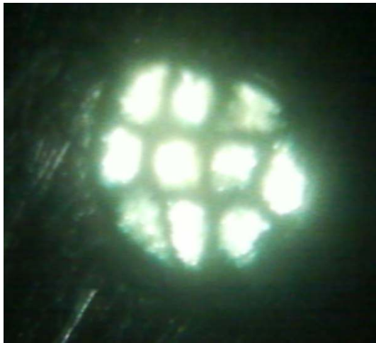
Fig. 5 A cross-sectional image of a yarn from denim fabric. Few yarns from a denim fabric were removed and viewed under an optical microscope with a magnification of \times 50 . Ring dyeing can be seen through the cross-sectional image
