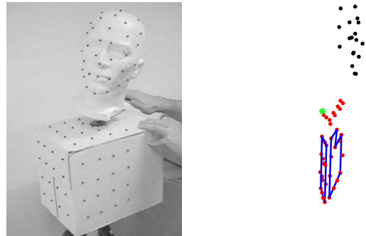
Figure 9. The left image shows a frame from a sequence with two articulated bodies with a universal joint. The right image shows the overall 3D reconstruction which has wrong depth estimates.
