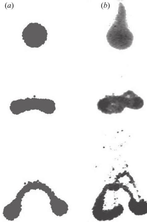
FIGURE 2. Typical evolution of a cloud in the macro-scale-inertia regime: (a) the simulations of Bosse et al. (2005a,b) with Re_c = 1 , N_0 = 10\,0096 and \ell^* = 2600 and (b) the experiment with Re_c = 0.7 , N_0 = 16\,000 and \ell^* = 179 ( Re_p = 8 \times 10^{-5} , R_0/a = 66 , \phi = 6\% and St = 2 \times 10^{-5} ). The complete dynamics for the experimental case is shown in supplementary movie 1 (available at journals.cambridge.org/flm ). The movie of the numerical simulation can be seen in Bosse et al. (2005a). The upward tail of the experimental cloud at initial time is due to the injection process.
