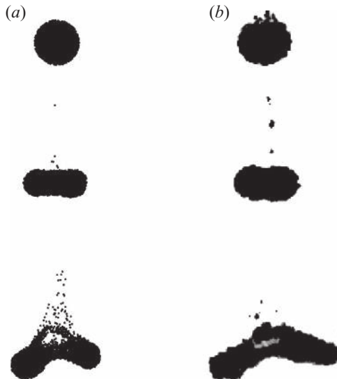
FIGURE 4. Typical evolution of a cloud in the micro-scale-inertia regime for \ell^* \approx 20 : (a) the Oseenlet simulations with N_0=7500 and \ell^*=20 and (b) the experiment with Re_c=3.5 , N_0=7000 and \ell^*=21 ( Re_p=2 \times 10^{-3} , R_0/a=24 , \phi \approx 50\% and St=5 \times 10^{-4} ). The complete dynamics for the experimental case is shown in supplementary movie 3 and for the Oseenlet simulation in supplementary movie 5.
