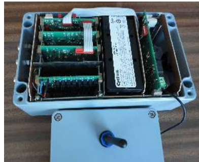
Fig. 6. View of internal construction of the analyzer with wireless communication.
