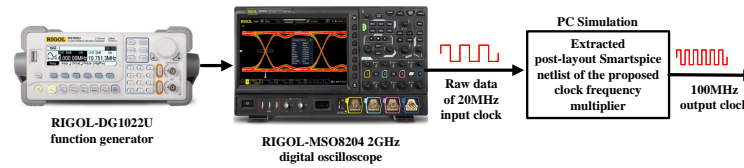
Figure 14. Simulation setup diagram of the proposed clock frequency multiplier.
