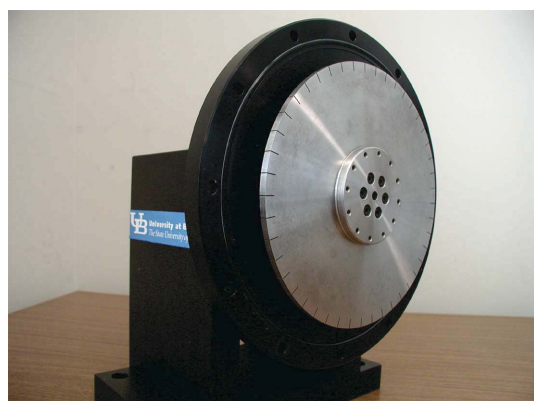
Figure 1 Shutter with partially dismantled vacuum chamber.
