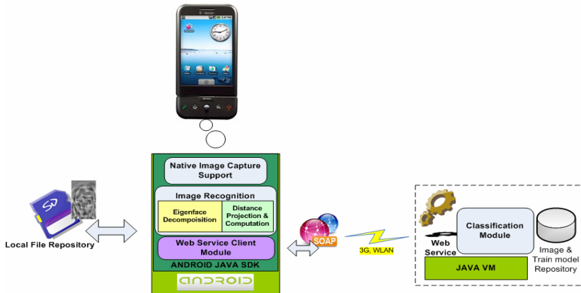
Fig. 2. Architecture of the proposed mobile face recognition system
