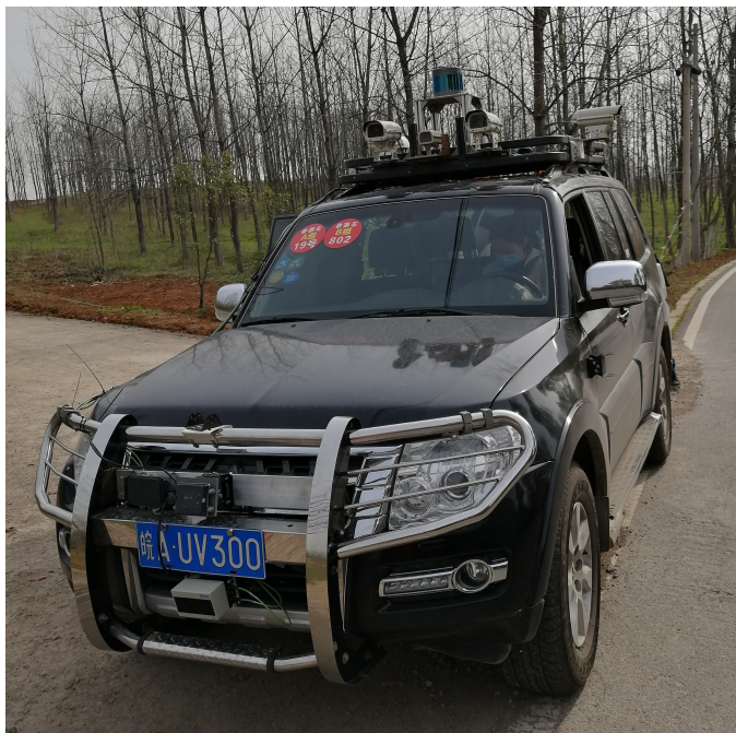
Fig. 19. ALV used for the experiments in various environments. It is equipped with cameras, lasers, and positioning sensors for perception.
