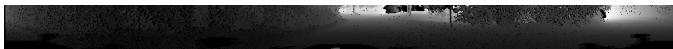
Fig. 8. Range image. The number of rows in the image is defined by the number of lasers in the LiDAR. The number of columns is given by the laser’s range reading of 360^\circ per rotation. The Velodyne HDL-64E, for example, has a range map width of about 1800 and a height of 64.
