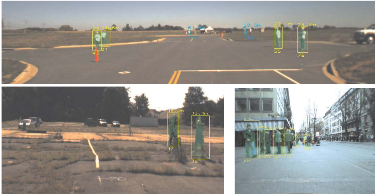
Fig. 1. Examples of test scenarios and the output of our pedestrian detection system (yellow boxes are detections with range and track ID text and a green overlay of the segmented person; the cyan boxes are missed detections).
