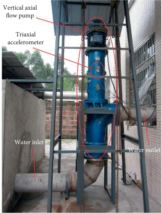
FIGURE 3: Experiment of vertical axial flow pump.
