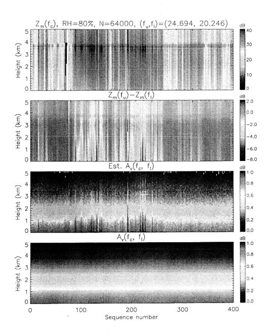
Fig. 2. Simulated fields of measured reflectivity factor at  $f_c=22.235$  GHz (top), differential measured reflectivity factor (second from top), estimated differential water vapor absorption (third from top) and assumed differential water vapor absorption (bottom). All units are in dB. ( $\gamma=0.39$ ).
