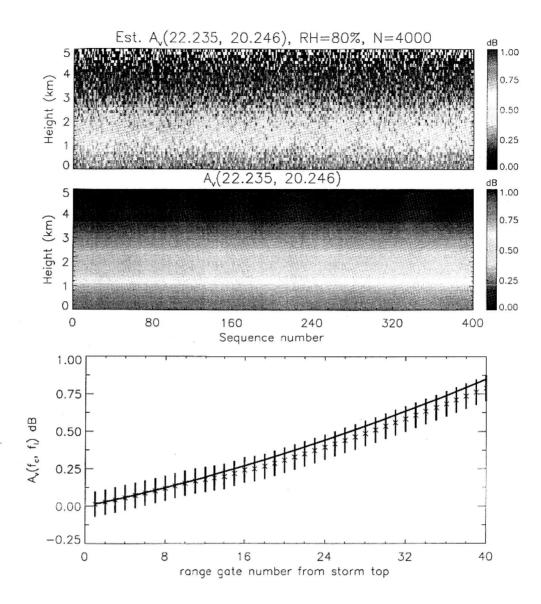
Fig.9. Estimated (top) and assumed (center) differential water vapor absorption; bottom: assumed (solid line) and the mean (X) and twice the standard deviation (vertical bars) of the estimates versus range gate number. A bandwidth of 20% is assumed with  $\gamma$ =0.42.
