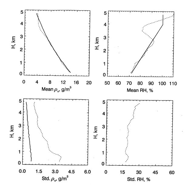
Fig.13. Top left: Mean profiles of estimated (dashed line) and assumed (solid) water vapor density versus height. Top right: Mean profiles of estimated (dashed line) and assumed (solid) relative humidity, RH. Bottom left: Standard deviation of estimated (dashed line) and assumed (solid) water vapor density. Bottom right: Standard deviation of estimated (dashed line) relative humidity. n=16,000 and 20% bandwidth.
