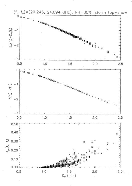
Fig.5. Measured (top) and 'actual' (center) differential reflectivity factor and differential path attenuation (bottom) for a range gate in the snow just above the melting layer versus median drop diameter of melted particles,  $D_0$ .
