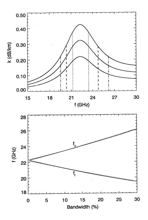
Fig.1. Top: Specific absorption of water vapor (dB/km) for water vapor densities  $(g/m^3)$  of 8.75 (lowest), 13.15, 17.5 (highest) and the frequencies at which the absorption is equal for bandwidths of 10%, 20% and 30%. Bottom: Upper and lower frequencies giving equal water vapor absorptions versus percent bandwidth. Solid lines represent numerical values; dashed lines represent quadratic approximations given by (8) and (9).
