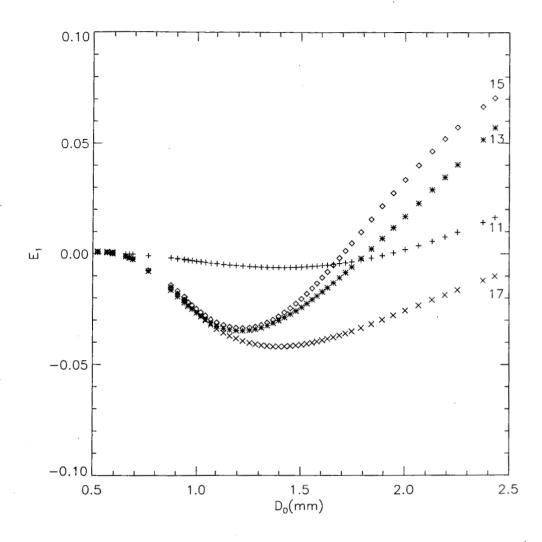
Fig.7. Bias term  $E_1$  for four range gates (11, 13, 15, 17) within the melting layer versus median mass diameter of the equivolume raindrops.
