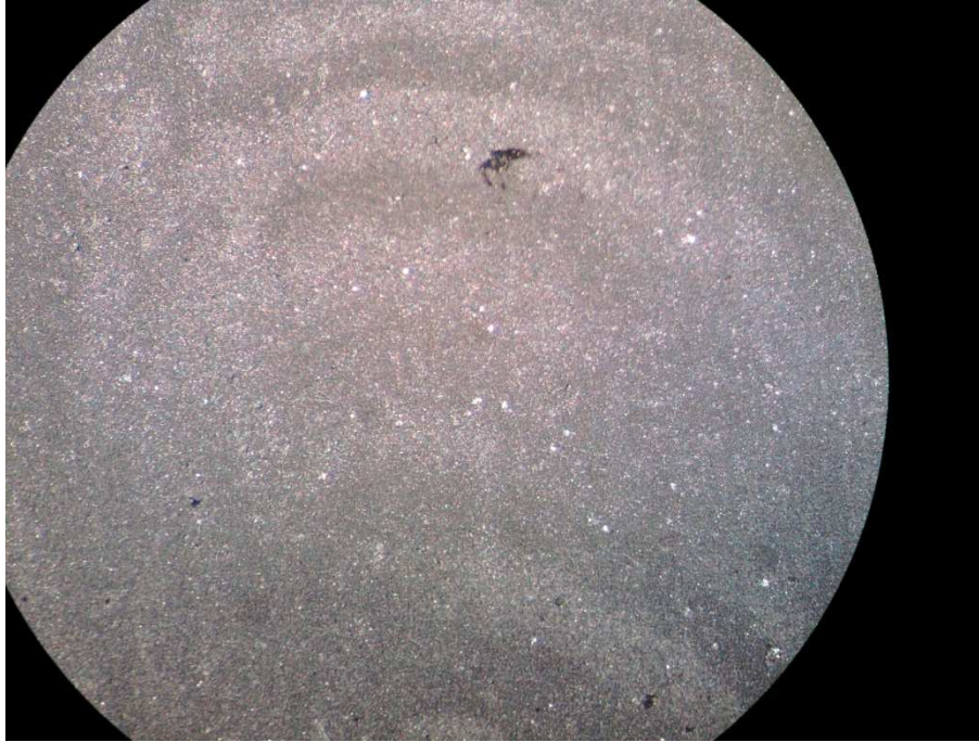
Figure 3.7: Photo of a silicone sample, taken through an optical microscope.
