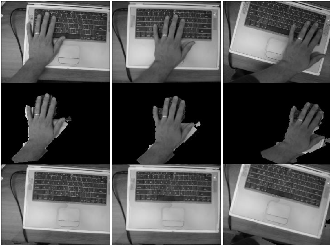
Figure 19: Illustration of video object deletion. (1) Original frames of size 180 \times 240 . (2) Segmented layer corresponding to the motion of the hand. (3) Reconstruction without the hand layer using the recovered motion of the keyboard. Note that no additional frames beyond the three shown were used as input.
