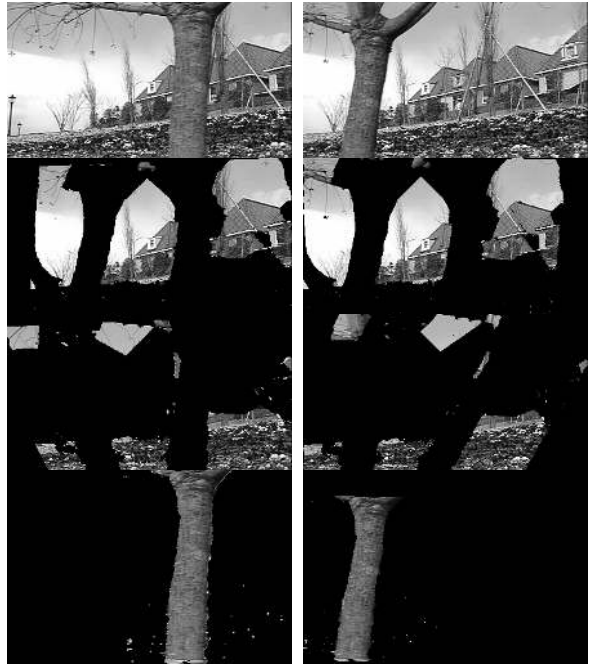
Figure 8: Flower Garden sequence. (Row 1) Original image pair of size 240 \times 360 , (Rows 2-4) Pixels assigned to warp layers 1-3 in I and I' .
