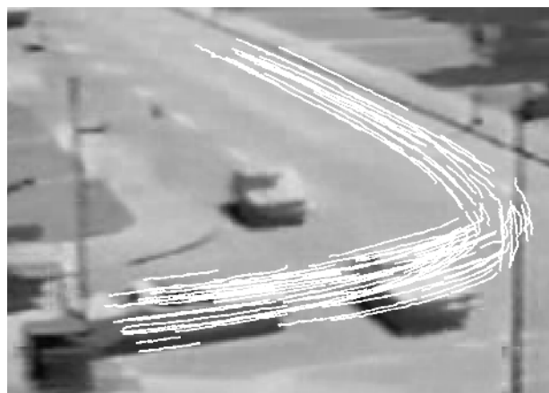
Figure 3: Illustration of feature tracking disruption as a vehicle is turning and its pose changes (displayed upon the frame of the first feature detection). However, the features are correctly grouped as one vehicle with our method.
