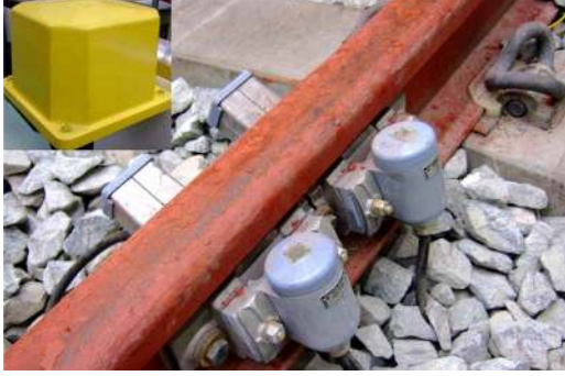
Fig. 2. Axle counter consists of two pairs of transmitter and receiver. Inset shows the track side converter equipment connecting the axle counter.
