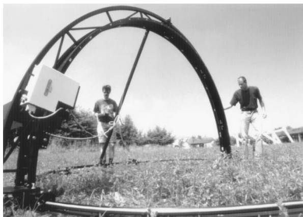
Fig. 1. FIGOS field goniometer assembled with the GER-3700 spectroradiometer for a field campaign at the University of Zürich campus.
