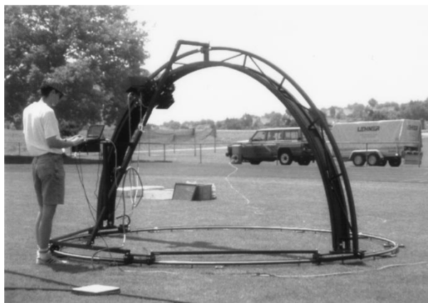
Fig. 3. Overview of FIGOS showing the PC control unit for the GER-3700 sensor (on the left), the spectralon reference panel (in the foreground), and the trailer used for transporting FIGOS (in the background).
