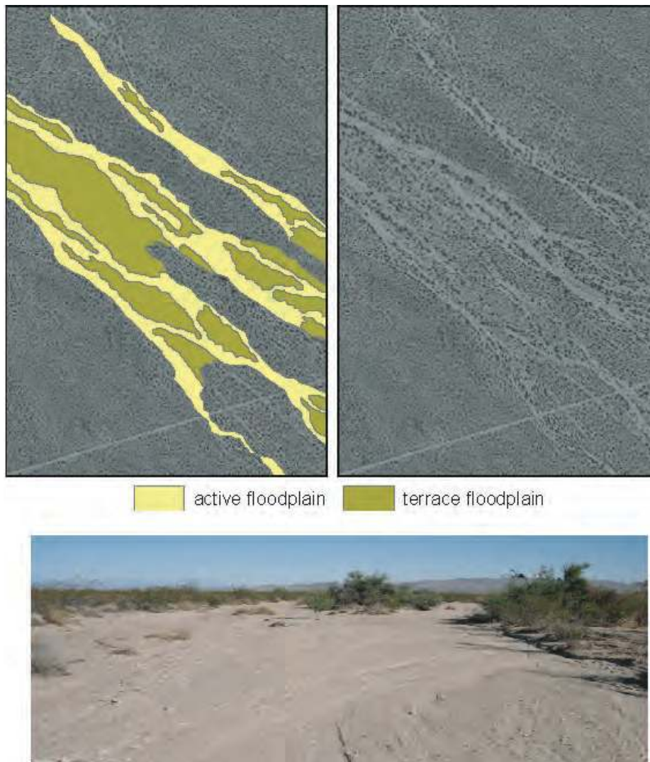
Figure 40. Example geomorphic mapping of a compound channel showing a mosaic of terraces within the active floodplain, Caruthers Creek, CA.
