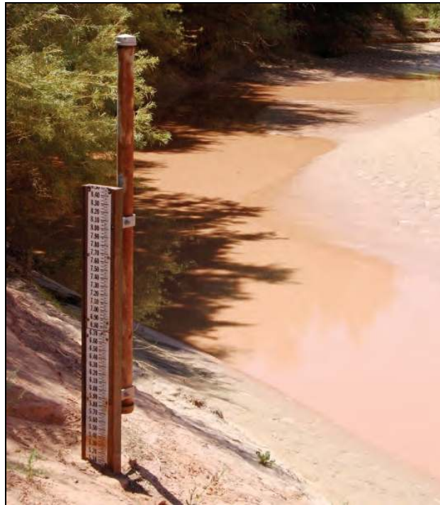
Figure 38. Staff used to determine stage height for Chinle Creek, AZ.
