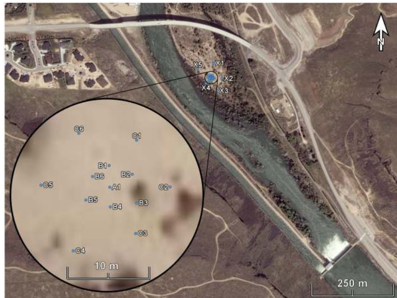
Figure 1. Map showing location of BHRS relative to Boise River. Inset shows geometric layout of wells in the central area of the site. Diversion Dam, which controls river levels, can be seen in lower right.
