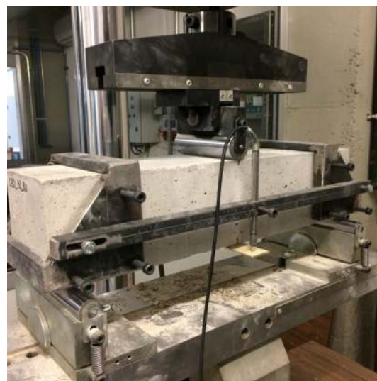
Fig. 5 Three-point bending test of a notched specimen according to the RILEM work-of-fracture method.
