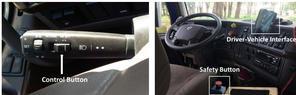
Figure 1. The CACC control stalk (left) and truck cockpit interior (right) with driver-vehicle interface (DVI) and safety button.
