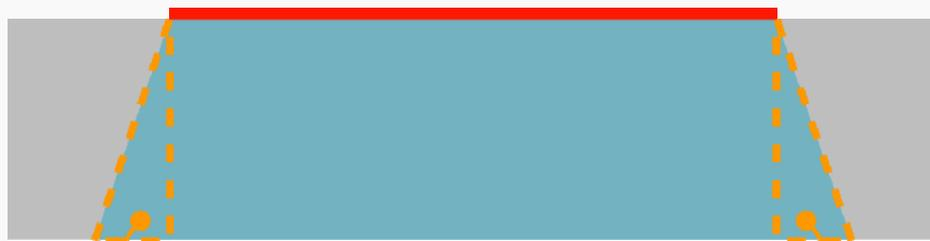
bar shaped body with approx. 1-D heat flow
