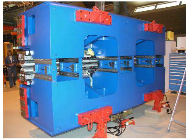
FIGURE 2. Front and back side of the fixed gap UE44. The support structure is a heavy, but simple and stiff welding construction.
