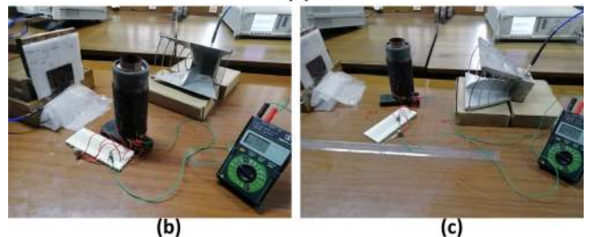
FIGURE 15. Description of the overall structure and measurement setup (a) closed view of cylindrical rectenna. Measurement setup for the fabricated rectenna array (b) both transmitting antennas are at 90° to each other (c) once the transmitting Horn antenna and fabricated monopole antenna are in line of sight.
