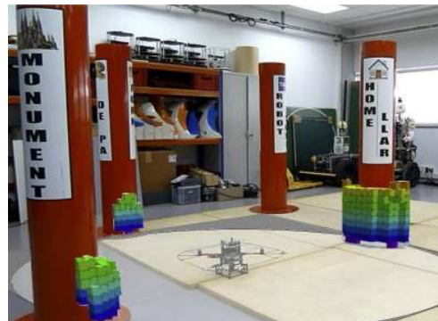
(b) Overlapping of the real and simulated environments with the Octomap containing the detected obstacles (coloured Voxels) and the sensing area (white circle with an alpha channel reduction).
