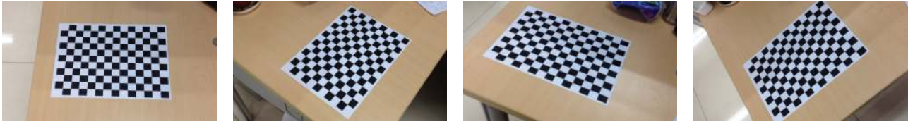
FIGURE 11: Four images of model plane for camera calibration.
