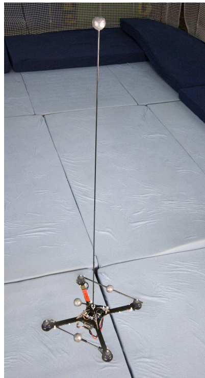
Fig. 3. The quadrotor balancing the pendulum, at standstill. The mass center is about half-length of the pendulum.
